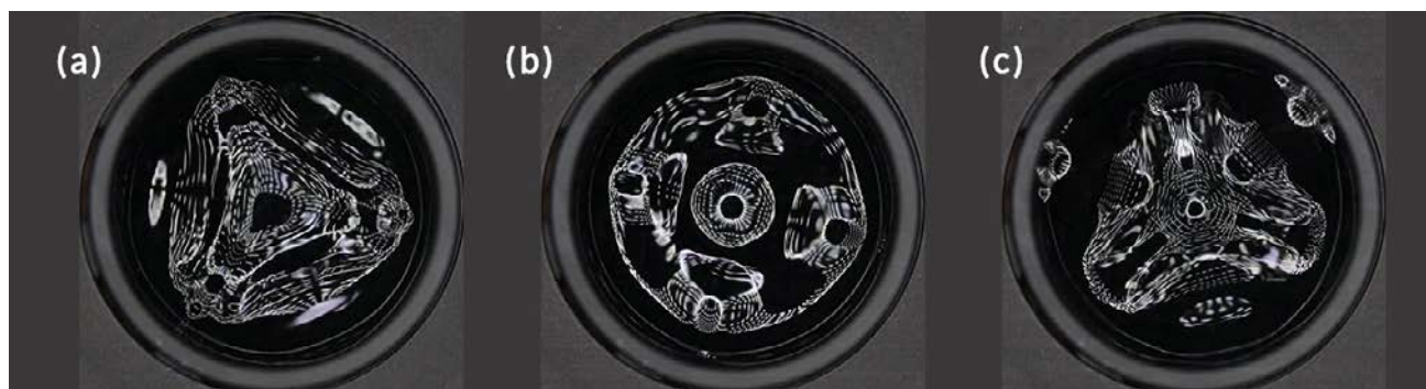
Figure 34. A cymaglyph observed in a circular cuvette at: (a) a frequency of 26.5 Hz ; (b) the corresponding 4:3 (perfect 4th) ratio frequency of 35.34 Hz ; and (c) both frequencies 26.5 and 35.34 Hz , resulting in an interference cymaglyph showing the dominant characteristics of the 26.5 Hz frequency pattern.
