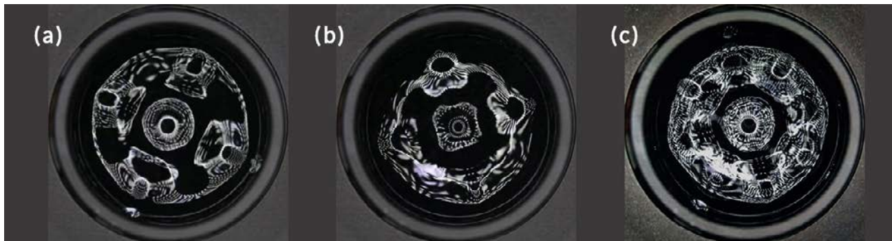
Figure 25. A series of unstable cymaglyphs from a circular cuvette at a frequency of 35.34 Hz showing: (a) 4-fold symmetry; (b) the opposite 4-fold symmetry; and (c) the composite 8-fold symmetry.
