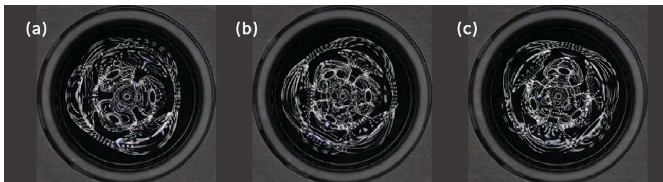
Figure 28. A series of cymaglyphs showing counterclockwise rotation in a circular cuvette at a frequency of 74.76 Hz . We can see at a time of: (a) 7 seconds, the reference point; (b) 13 seconds, a rotation of approximately 45 degrees; and (c) 18 seconds, a further rotation of 45 degrees.
