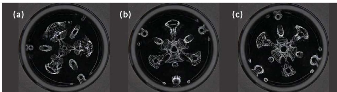
Figure 29. A series of cymaglyphs showing clockwise rotation in a circular cuvette at a frequency of 26.5 Hz . We can see at a time of: (a) 7 seconds, the reference point; (b) 9 seconds, a rotation of approximately 30 degrees; and (c) 18 seconds, a further rotation of 30 degrees.
