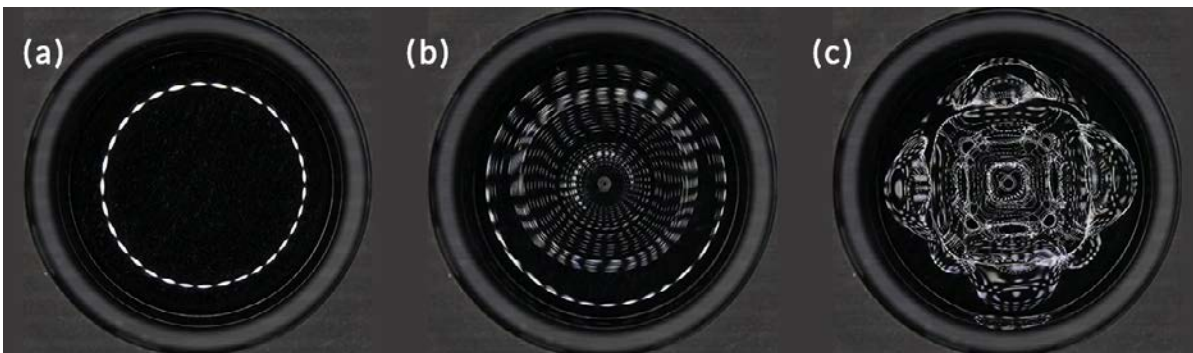
Figure 18. Ring patterns in a circular cuvette at a frequency of 64 Hz, showing: (a) one ring pattern of 32 dashes corresponding to the 32 diodes in the CymaScope light ring; (b) concentric rings due to an amplitude increase; and (c) the 4-fold pattern formation after sufficient (critical) amplitude has been applied.
