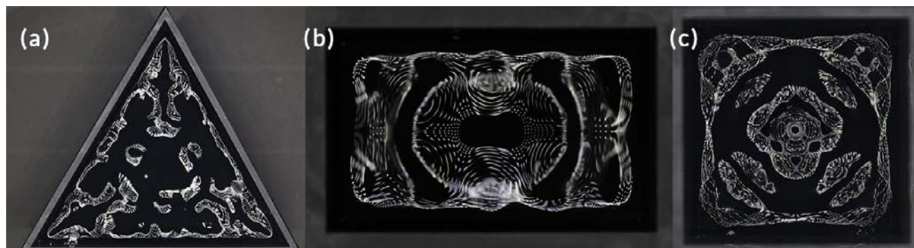
Figure 17. Cymaglyphs showing different symmetry folds for: (a) a triangular cuvette at a frequency of 45 Hz showing 3-fold symmetry; (b) a rectangular cuvette at a frequency of 36 Hz showing 2-fold symmetry; and (c) a square cuvette at a frequency of 89 Hz showing 4-fold symmetry.
