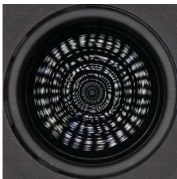
Figure 19. Cymaglyph showing concentric rings in a circular cuvette at a frequency of 183.428 Hz.
