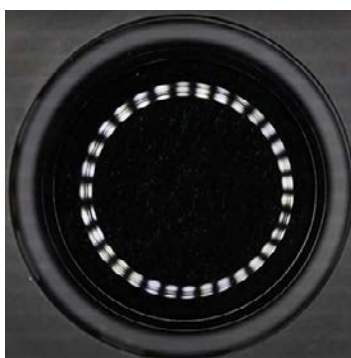
Figure 13. Pre-cymaglyph from a circular cuvette at a frequency of 214 Hz.
